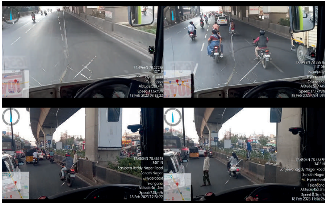
Figure 2.3 ADAS unit alerts driver with unsafe distance warning for VRUs; Pedestrians and Vehicles, including 2-wheelers are detected; FCW, HMW, LDW, and PCW.
