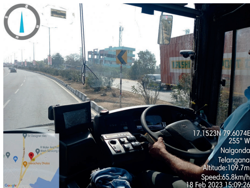
Figure 2.2 ADAS-enabled bus; the main components of an ADAS devices such as CAS and DMS include a camera unit focused on the road and a display unit.
